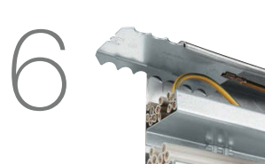
6 Special sheet-metal couplings provide mechanical and electrical joining of the bottom trunking part.
